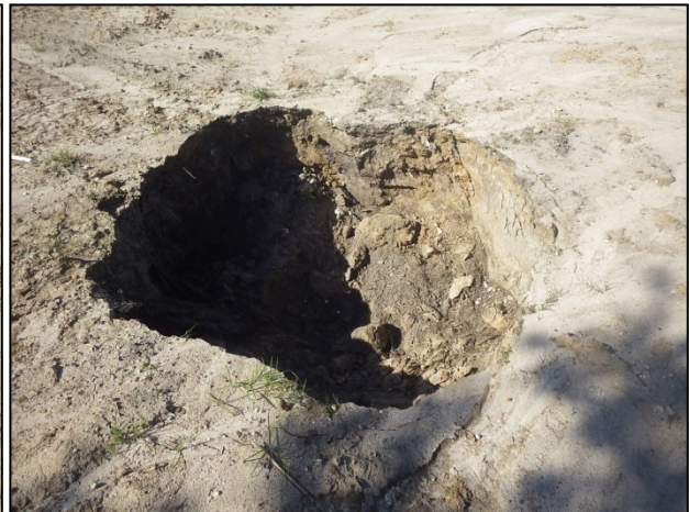
Figure 14: Image of sinkhole "C" that has 3.2 and 3.0 m diameters and a maximum depth of 1.4 m (Latitude 29°40'47.69"N / Longitude 82°29'43.25"W).
