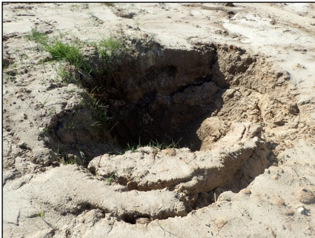
Figure 13: Image of sinkhole "A" that is 3 m in diameter with a maximum depth of 1.5 m (Latitude 29°40'47.99"N / Longitude: 82°29'42.99"W).
